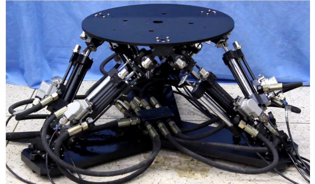
L. Cui, et al., Six Degree-of-freedom Hydraulic Hexapod Platform for Large-amplitude Vibration Isolation, 11th International Conference on Control Automation and Systems, 2011
